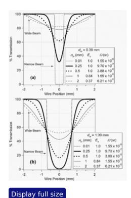
For an extremely broad (nearly uniform) beam of particles the attenuation is simply the geometric area of the vaporizer that the wire probe is blocking (because the particle probability density is nearly uniform across the width of the vaporizer). For particle
