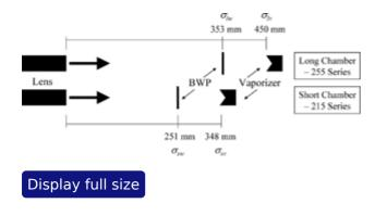
TABLE 1 Particle flight distance, vaporizer (or laser spot) size, and solid angles of collection for the detection geometries of the long-chamber and short-chamber AMS, and two laser ablation particle mass spectrometers (Cziczo et al. 2003; Gard et al. 1997). The solid angle of detection represents the geometric area sampled by the vaporization laser or vaporizer at the given particle flight distance from the lens exit
