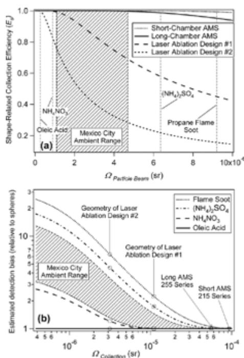
This increase in estimated detection bias arises from the fact that laser spot sizes are small, leading to relatively smaller solid angle of detection. The percentage of particles collected from a wide beam, therefore, is also small, and detection is sensitive to the particle beam width. The AMS has an advantage in this regard, because of its relatively large solid angle of collection, due to its large vaporization surface ( $d_v = 3.81$  mm) as compared to typical laser spot sizes.
